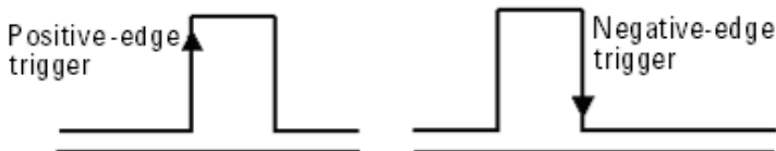
Figure4-11 Positive and negative edge of digital trigger.
